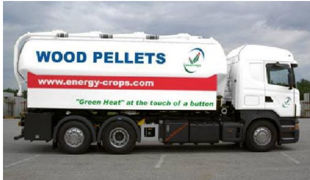
Fig 8 Tanker with on-board weighing system – delivery to storage bunker 14
