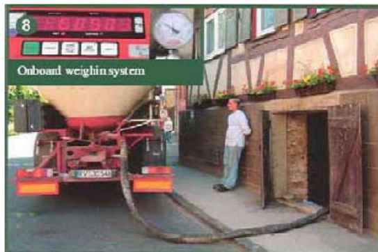
Fig 8 Tanker with on-board weighing system – delivery to storage bunker 14
