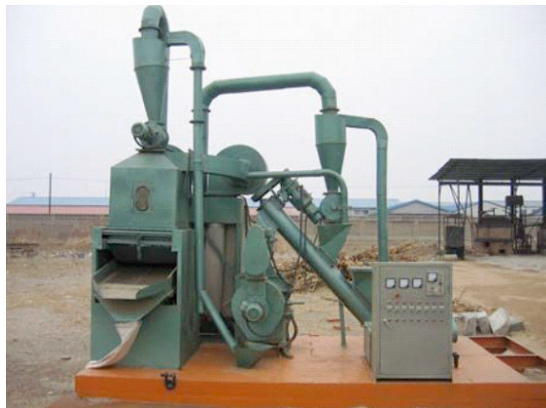
Fig 32 Greenforze Mobile pellet line - EkoPell Micro Factory 250
